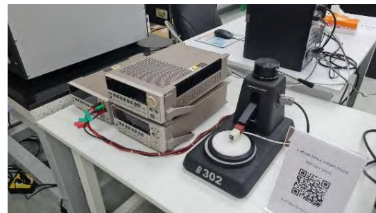
Figure 5 Source meter unit instrument (Keithley 2410) with a Linear 4-Point Probe
